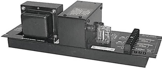
The GE Model 110-3693 AC Clock Power Supply provides a convenient 24Vac source for operating synchronous clocks and bells. The low voltage and current output of this power supply allows Class 2 wiring to be used. An onboard relay allows clock correction coils to be easily interfaced with GE master clocks. This supply mounts with the standard GE power supply backbox and doors.
